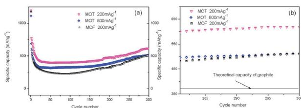
**Fig. 3** Variation in discharge capacity vs. (a) cycles and (b) the last 20 cycles of MOT at different current densities of 200 and 800 mA g<sup>-1</sup>, and that of MOF at a current density of 200 mA g<sup>-1</sup>.
