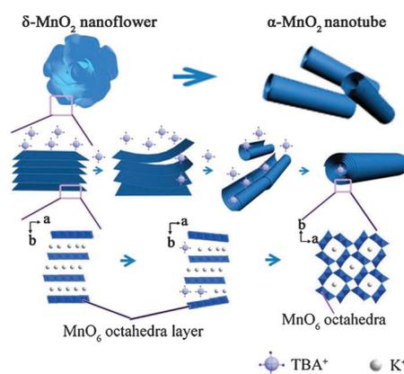
**Fig. 2** Scheme of evolution from nanoflower to nanotube  $\text{MnO}_2$  via an exfoliation and self-scrolling process.
