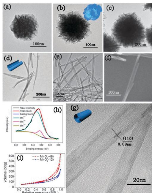
**Fig. 1** Morphology evolution of  $\text{MnO}_2$  from nanoflowers to nanotubes with different reaction times: TEM images of the products obtained for (a) 1, (b) 6, (c) 12, (d) 24 and (e) 48 h and (f) SEM after 48 h; (g) HRTEM image and (h) the fitted XPS spectra of  $\text{Mn } 2p_{3/2}$  for the product at 48 h; (i)  $\text{N}_2$  adsorption/desorption isotherms of products at 12 and 48 h.
